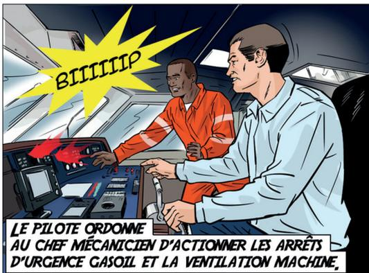
LE PILOTE ORDONNE AU CHEF MÉCANICIEN D'ACTIONNER LES ARRÊTS D'URGENCE GAZOIL ET LA VENTILATION MACHINE.
