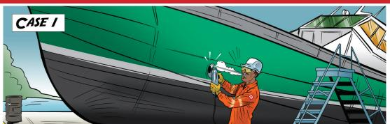
A painter used a defective angle grinder during a maintenance operation. After a few minutes of use, the disk, which was unsuitable for the operation, shattered and struck his face.
