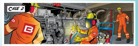
During an oxy-cutting operation in the engine room of a Crewliner, the acetylene hose from the welding station broke free of the torch and began shooting out flames. The welder rapidly cut off the gas.
