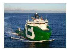
Extremely versatile, she can perform numerous tasks in addition to anchor-handling, such as supply duties, oil recovery, standby operations, firefighting, rescue (up to 300 survivors) and ROV operations. With a strengthened hull and enhanced winterization equipment (Ice class), she is perfectly suited for work in temperatures down to -20° C while ensuring maximum safety conditions.
