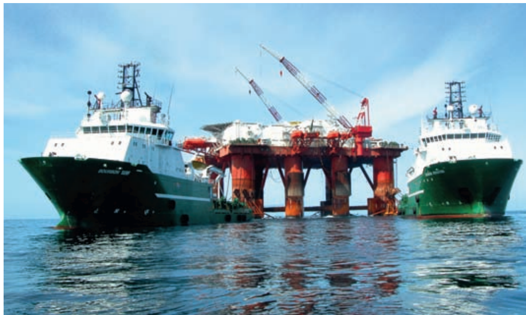
> Above The Kakulo, a tug used for assistance and operations on offshore oil and gas terminals. > Right The AHTS Bourbon Surf and Bourbon Borgstein, by a semi-submersible platform in the North Sea.
