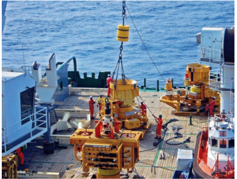
> Preparation for launch of a subsea package (Xmas tree and well head).
