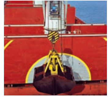
> Start of coal unloading operations by 13 m 3 "Peina" buckets onboard the Shangor.
