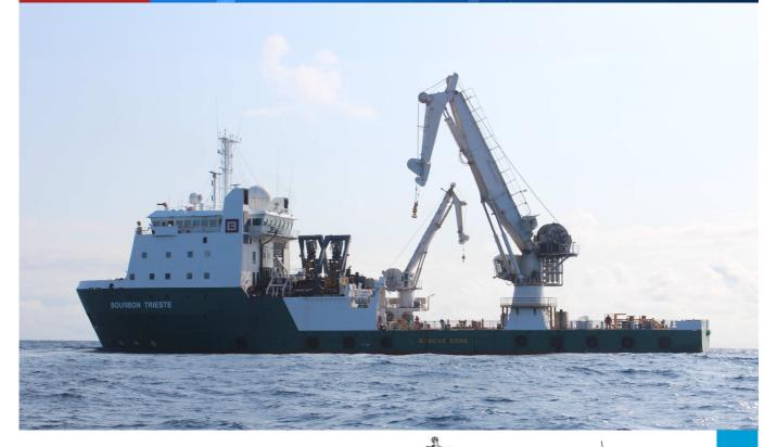
BOURBON TRIESTE is a De Hoop design, diesel electric, DP 2, multipurpose subsea services support vessel with twin deepwater offshore cranes and accommodation for 70 persons.
