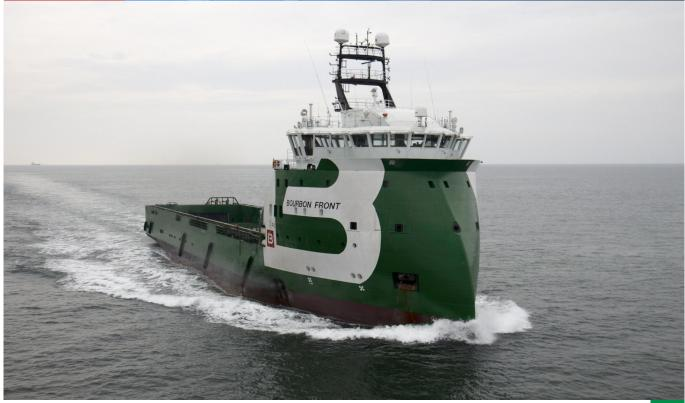
The BOURBON RAINBOW is a large platform supply vessel designed to meet the future demands of the offshore industry. The hull with ULSTEIN X BOW combined with diesel-electric propulsion systems ensure outstanding performances with regards to fuel consumption, sea-keeping, station-keeping, speed and cargo capacity.
