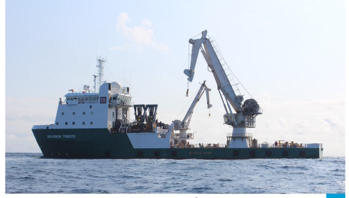
BOURBON TRIESTE is a De Hoop design, diesel electric, DP2, multipurpose subsea services support vessel with twin deepwater offshore cranes and accommodation for 80 persons.
