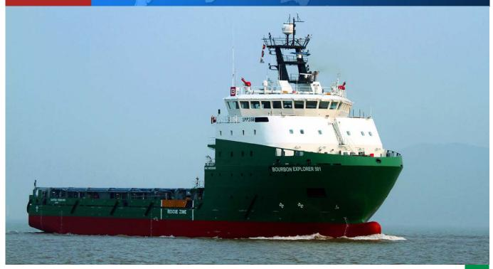
**BOURBON EXPLORER 500 Series - PSV** has been designed by Shanghai Design Associate. This extremely maneuverable vessel is equipped with Diesel Electric propulsion, four main engines configuration, 2 azimuth Z-drive at stern, two bow thrusters, and Dynamic Positioning Class II. It is capable of safe, reliable operations as well as precise stationkeeping in DP mode.
