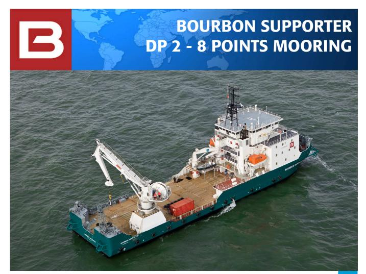
BOURBON SUPPORTER is a multipurpose subsea services support vessel, diesel electric, DP 2, equipped with an 8 points mooring system, one AHC deep water crane and accommodation for 103 persons.
