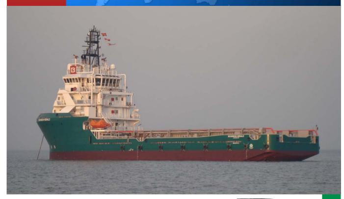
The BOURBON HORUS, a GPA 670 MkII ROV design was designed in conjunction with Guido Perla & Associates of Seattle, Washington. This environmentally friendly diesel electric vessel uses less fuel than conventional direct-drive propulsion vessels and produces far less pollution. The vessel is also classed DPII.
