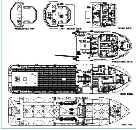
These anchor handling tug supply vessels were designed by CONAN WU to carry out general services for the offshore industry.
