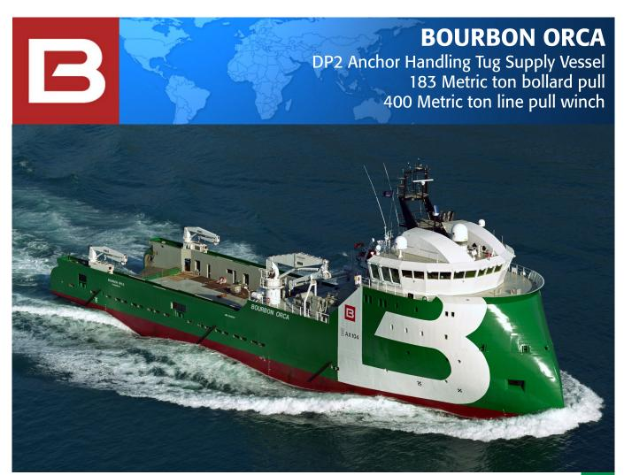
BOURBON ORCA, AX104-design from Ulstein Design is a Diesel electric AHTS with the patented Ulstein X-Bow. The vessel is equiped with 2 drums waterfall type for towing/working and 1 drum for anchor handling with large capacities, as well as 2 secondary drums. It is designed for World Wide service, for the purpose of performing and fulfilling the following duties:
