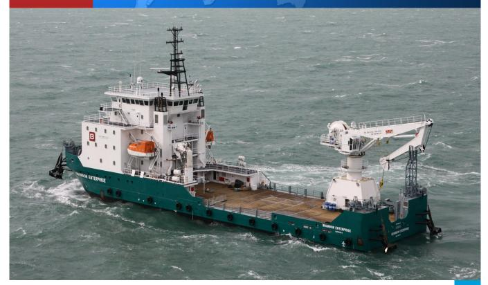
BOURBON ENTERPRISE is a Socarenam design multipurpose subsea services support vessel , diesel electric, DP 2, equipped with an 8 points mooring system, one AHC deep water crane and accommodation for 103 persons.
