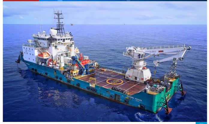
BAHTERA AZALEA is a multipurpose subsea services support vessel, diesel electric, DP 2, equipped with an 8 points mooring system, one AHC deep water crane and accommodation for 103 persons.
